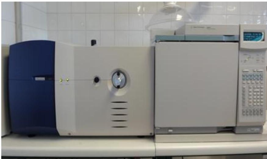
The GCT mass spectrometer with an analyzer time of flight (TOF) of orthogonal acceleration and high resolution (FWHM ~ 7000) is equipped with four sources of ionization.
