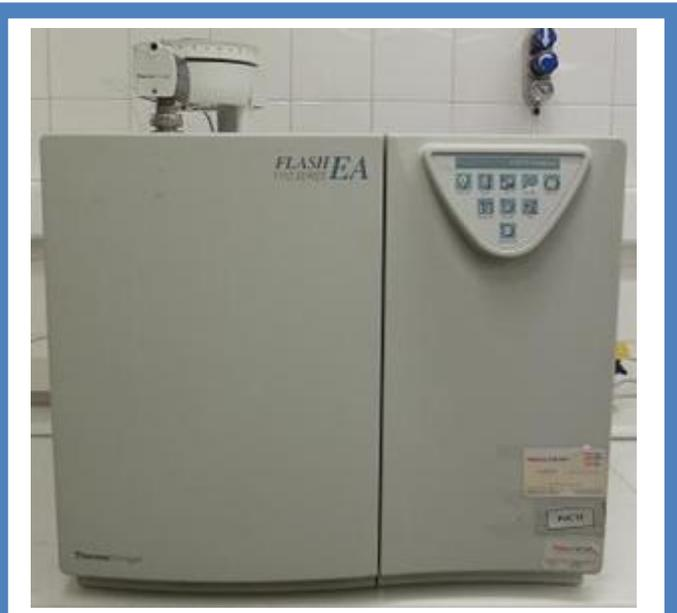
The analyzer operates on the basis of combustion dynamics of the sample. The sample is weighed into tin capsules and introduced into the combustion reactor using an automatic sampler, together with a certain amount of oxygen.
