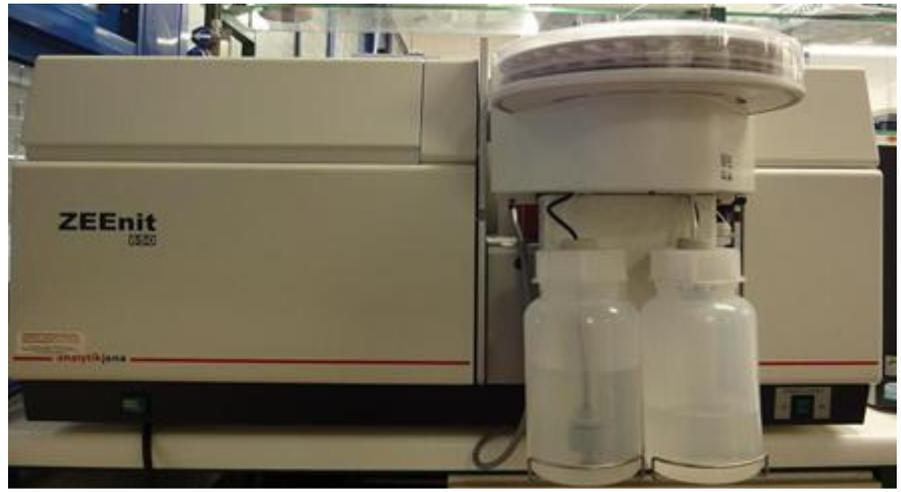
Graphite Furnace Atomic Absorption Spectroscopy is a highly sensitive spectroscopic technique that provides excellent detection limits for measuring concentrations of metals in aqueous and solid samples.
