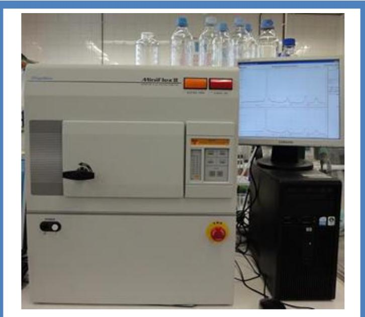
The powder X-ray diffraction (XRD) is one of the techniques used by mineralogists and solid state chemists to examine the physical-chemical make-up of solids. In this technique a diffraction pattern is obtained by registering the intensity of X-rays as a function of a scanning parameter (angle  $2\theta$ ).
