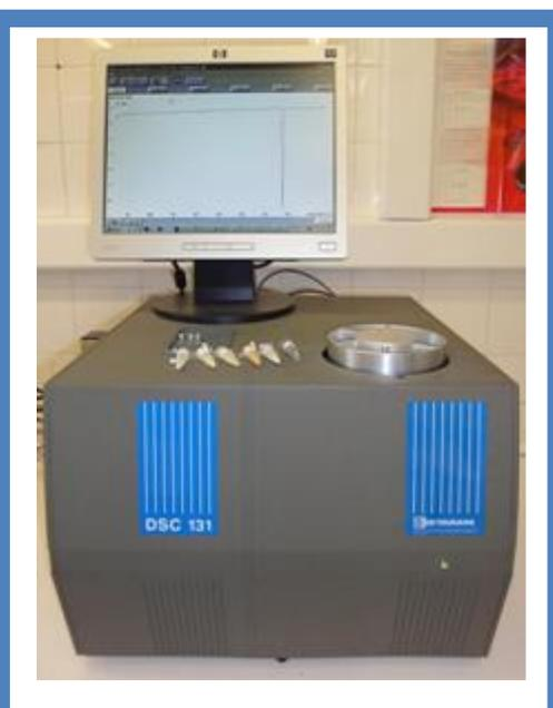
The differential scanning calorimetry (DSC) is a thermal analysis technique that records the flow of heat energy associated with transitions in materials as a function of temperature. This is a method of enthalpy variation, in which the difference in the supply of heat energy between a substance and a reference material is measured as a function of temperature, while both are subjected to the same program of heating or cooling, carefully controlled.
