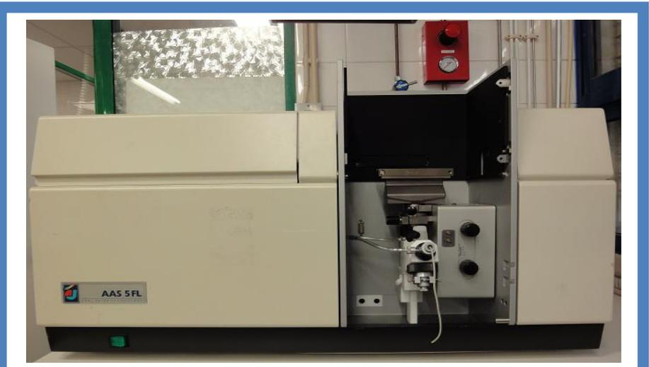
Flame Atomic Absorption Spectroscopy is a fast and easy technique with an extremely high sensitivity (particularly for elements like Pb, Cd, Cu and Cr). The sample is atomized in the flame, through which radiation of a chosen wavelength (using a hollow cathode lamp) is sent. The amount of absorbed radiation is a quantitative measure for the concentration of the analyzed element.
